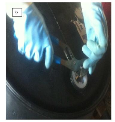
You need a piece of steel to fit between the wrench opening of plug and large channel lock pliers. Turn to the right and
