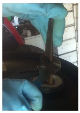
unscrew the plug. Insert the suction hose into barrel and fasten it as you saw in picture #6.
